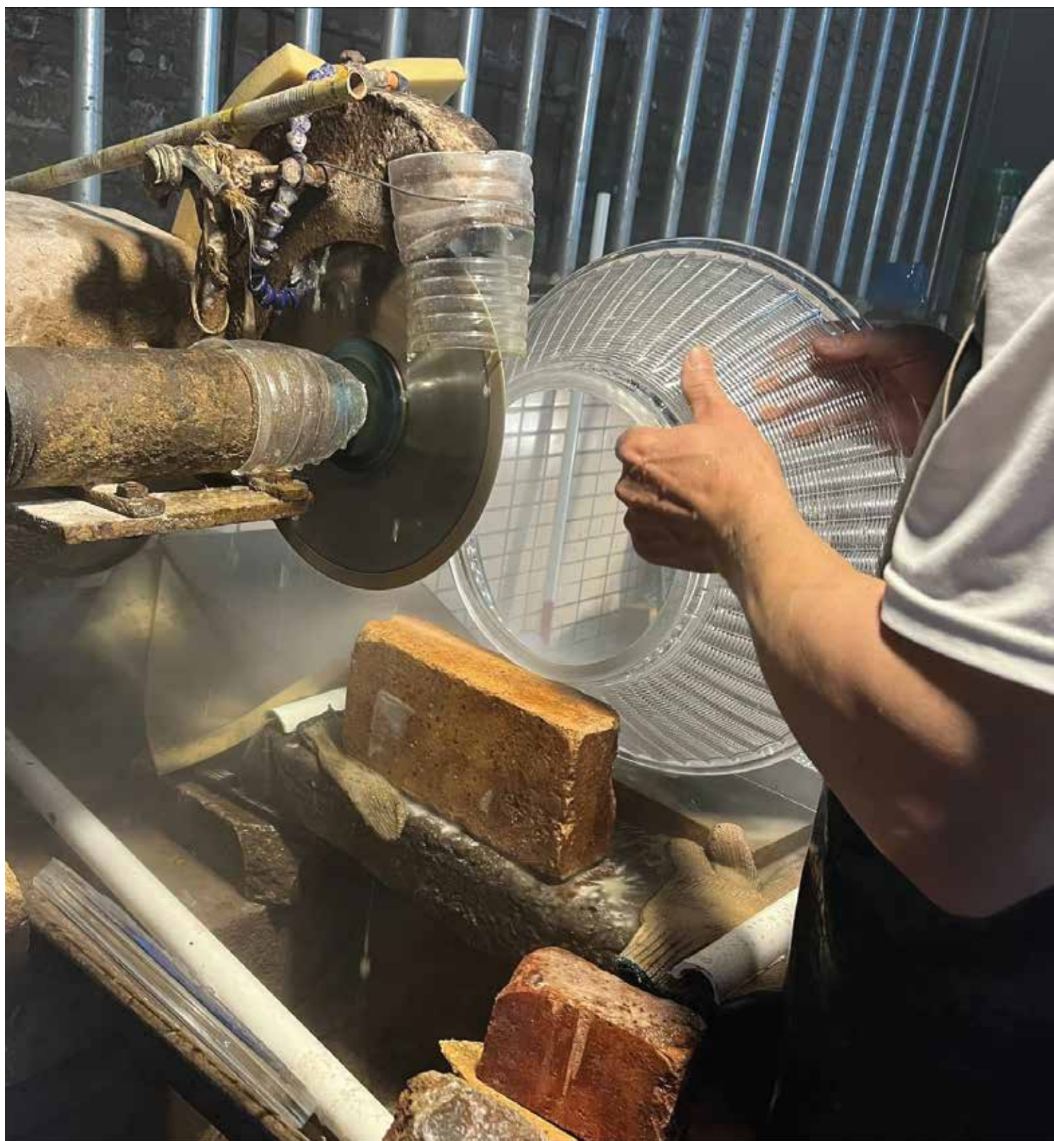
Fabrication of Custom Prismatic Soda Lime Glass Diffuser for Exterior Mounted Lantern
